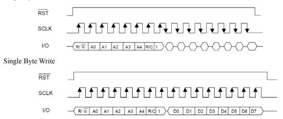
In burst mode, RST is kept high and additional SCLK cycles are sent until the end of the burst.
